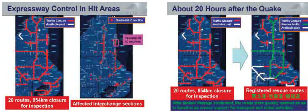
Figure 7.15: Return of NEXCO expressways back into service after the Great East Japan earthquake
