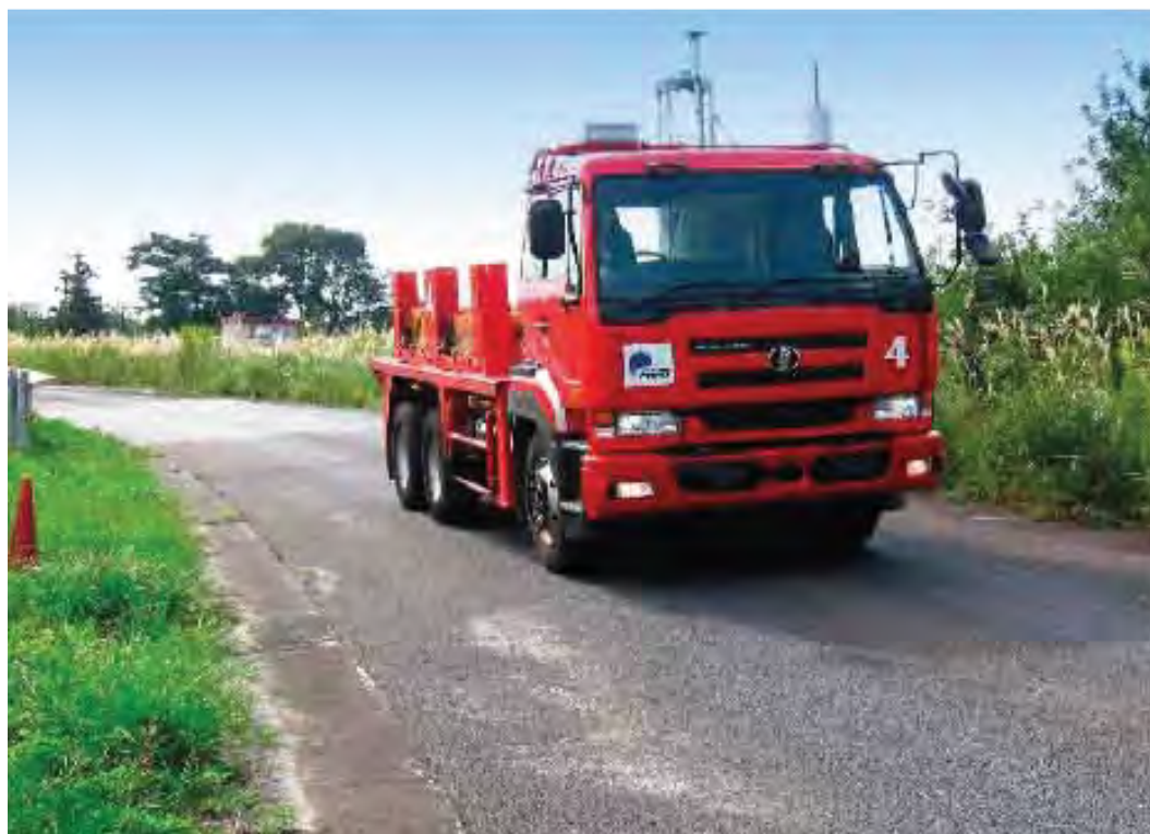
Figure B 1: Driverless vehicles used to track test pavements at PWRI research facility
