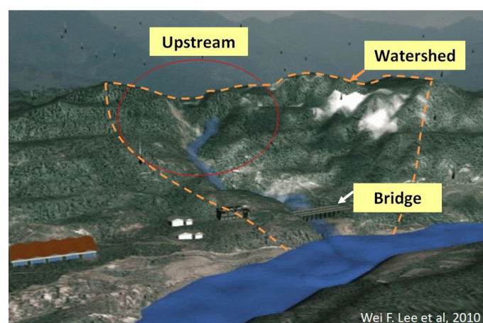
Figure 1: Schematic of watershed management for highway bridges
