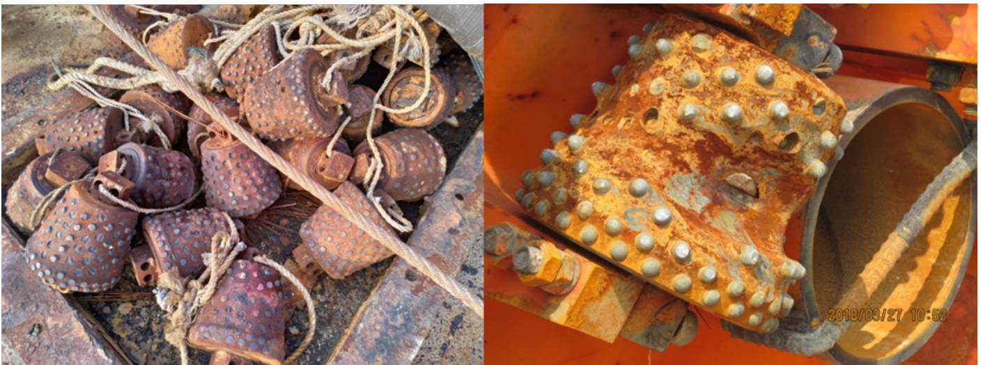
Figure 6: RCD Drill Bit Wear
