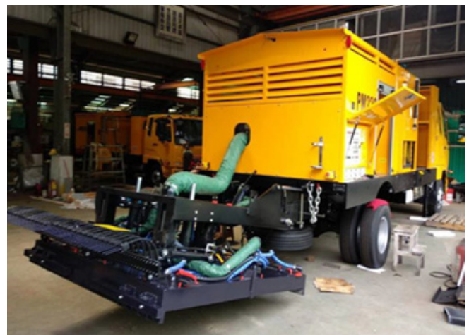
Figure 1: Hot-in-place recycling patching technology (a) Hand-push hot-in-place recycling patching machine; (b) Hot-in-place recycling repair unit
