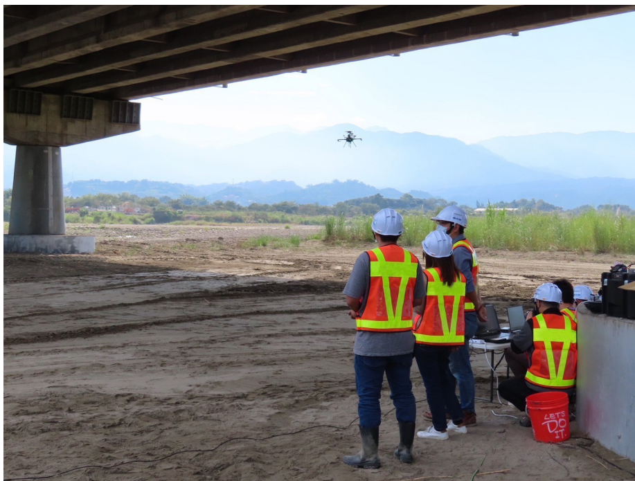
Using drones equipped with high-resolution cameras for bridge imaging
