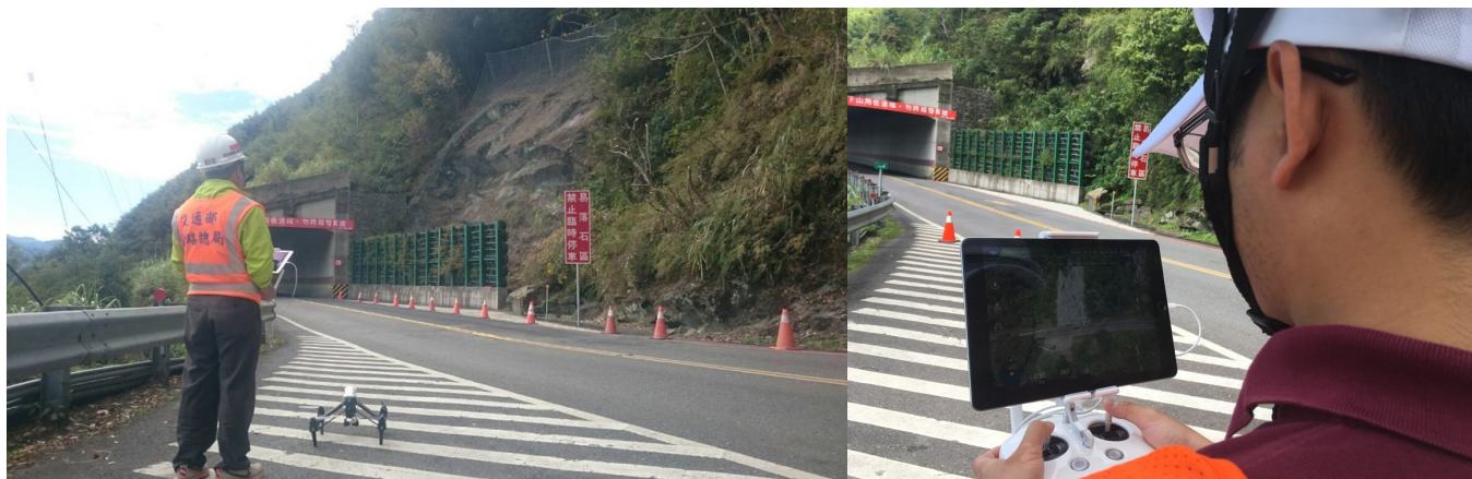
Real-time monitoring of highway slopes using drones
