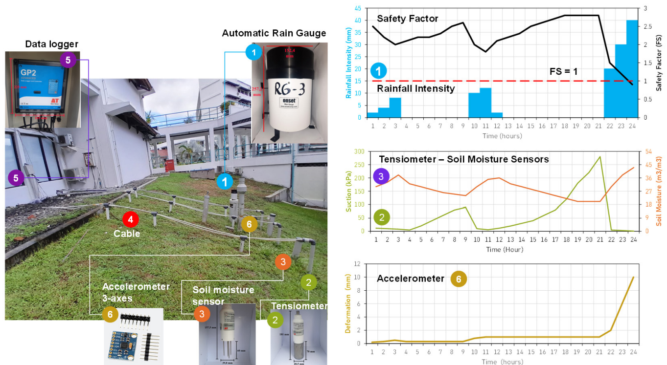
Figure 5: Traditional slope monitoring systems (Muntohar et al. 2024)
