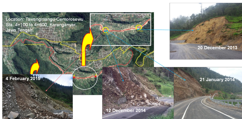
Figure 1: Debris deposit of the roadside slope failure: Tawangmangu-Cemorosewu road in Central Java
