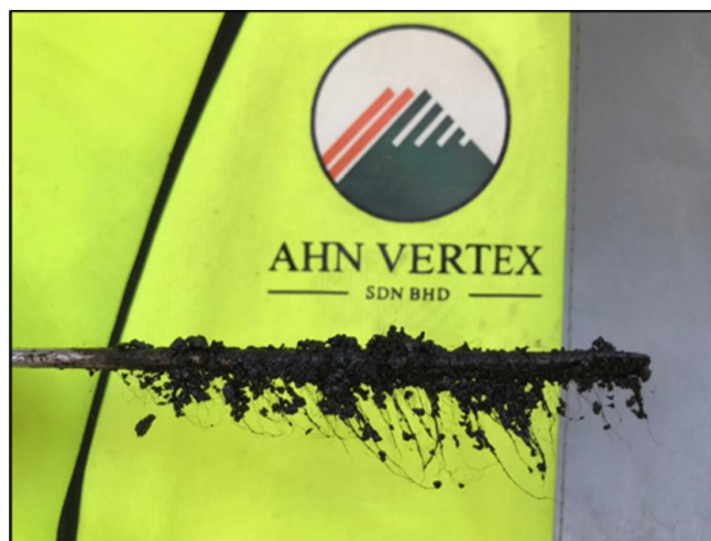
Figure 3: Distribution of fibre in SFM
