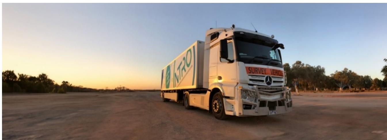
Figure 2: NTRO's Intelligent Pavement Assessment Vehicle (iPAVe) (Source: NTRO)
