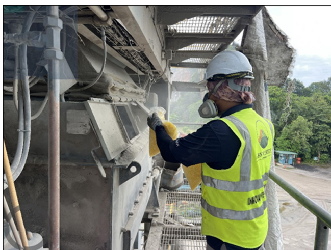
Figure 2: Mixing of SFM at batching plant
