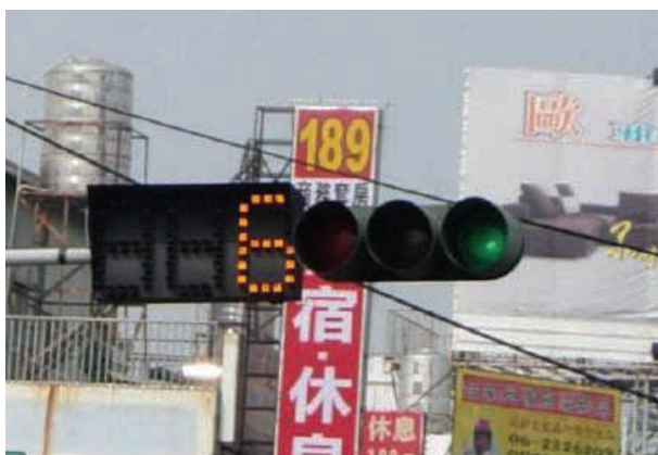
Figure 8.9: Plug in count-down monitor for green light (yellow number)
