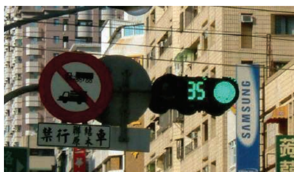
Figure 8.12: Built in count-down monitor for green light (green number)
