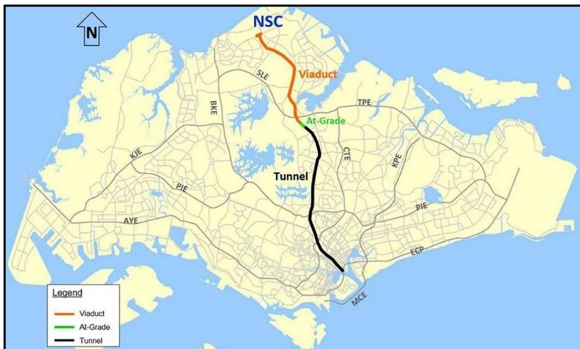
Alignment of North-South Corridor
