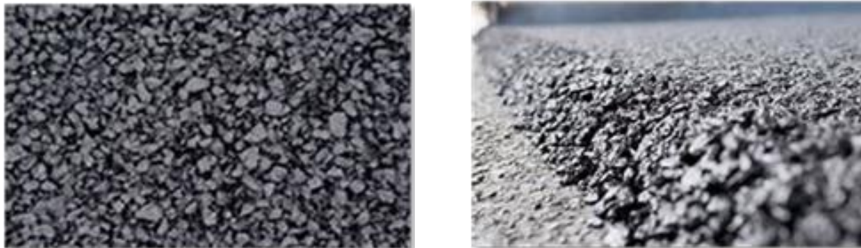
Figure 3-9: Stone mastic asphalt
